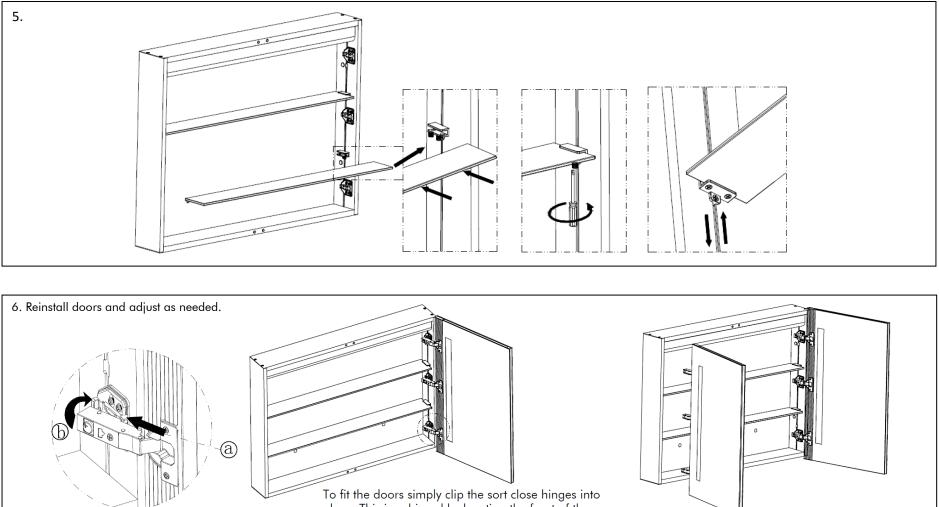
To fit the doors simply clip the sort close hinges into place. This is achieved by locating the front of the hinge into to cabinet mounting plate a ) and pushing in the rear of soft hinge until it clicks into place b ).
